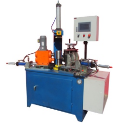
Three Stations Edge Trimming Machine (Cutting, Grinding and Curling)
